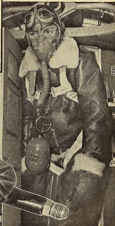
5. This crew member displays good sense by using the portable oxygen unit, known as the walk-around bottle, while moving about in a plane at high altitude. The equipment is used with the A-10 mask and provides a 4- to 8-minute supply of oxygen, depending on the altitude and the activity of the user.
